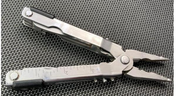
The main features of this Multi-Tool is that it has all the tools that I use on a daily basis and it collapses down to the small, compact form that fits on my belt. It is made of stainless steel and doesn't rust but is still magnetic enough so it will work with other magnetic tools. It contains 18 different tools as well as the ability to add bits to the Phillips head screw driver and blades to the saw blade holder.
