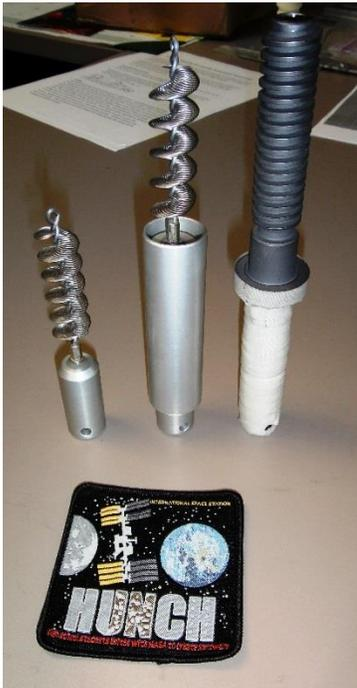
In the coming months NASA plans to change out all of the batteries that store the electricity coming from the solar panels due to their age. The bolts and nuts holding these batteries to the station have the potential to jam. The brushes built by the HUNCH students will get used to clean out and lubricate the nuts if there is a jam.
