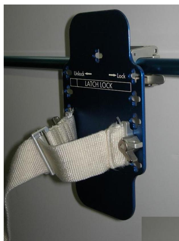
Short Duration Foot Restraint has 2 perpendicular configurations but no swiveling or pivoting capability.
