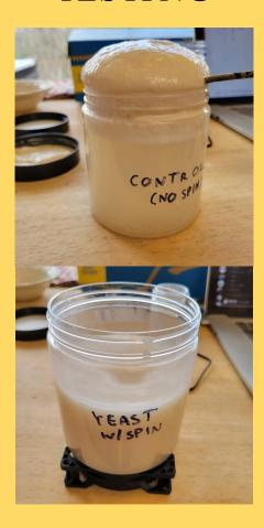
Multiple samples were tested to see how fermentation acts with our design. The control was not spun at all and led to a high degree of foam. The second sample was spun with the magnetic pill and led to far less foam. The final sample was spun with a closed lid to prevent oxygen from getting into the system.
