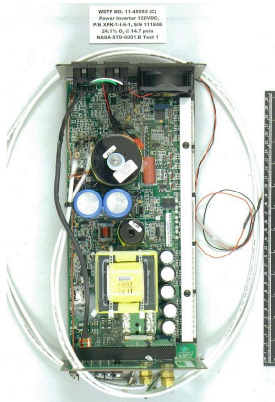
b. Internal view, case removed after test
