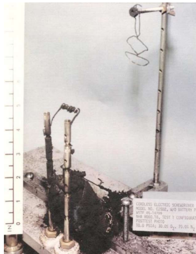
b. Posttest, no aluminum tape
