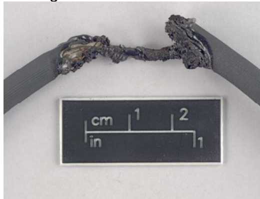
b. Damaged section of vacuum cleaner cable
