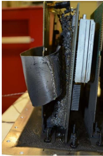
b. Posttest (burned internal electronics and foam)
