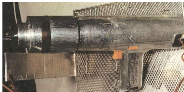
c. Protected by 3-mil aluminum tape
