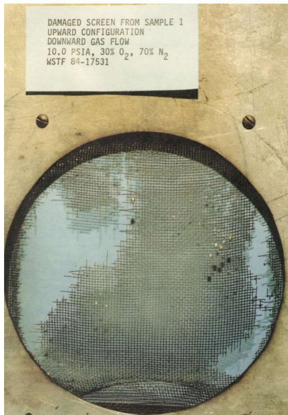
Figure 11. Damaged Aluminum Vent Screen from Airflow Tests
