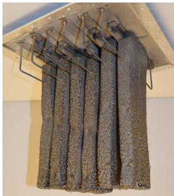
c. Posttest (burned foam -- 80% free volume, 20% foam)
