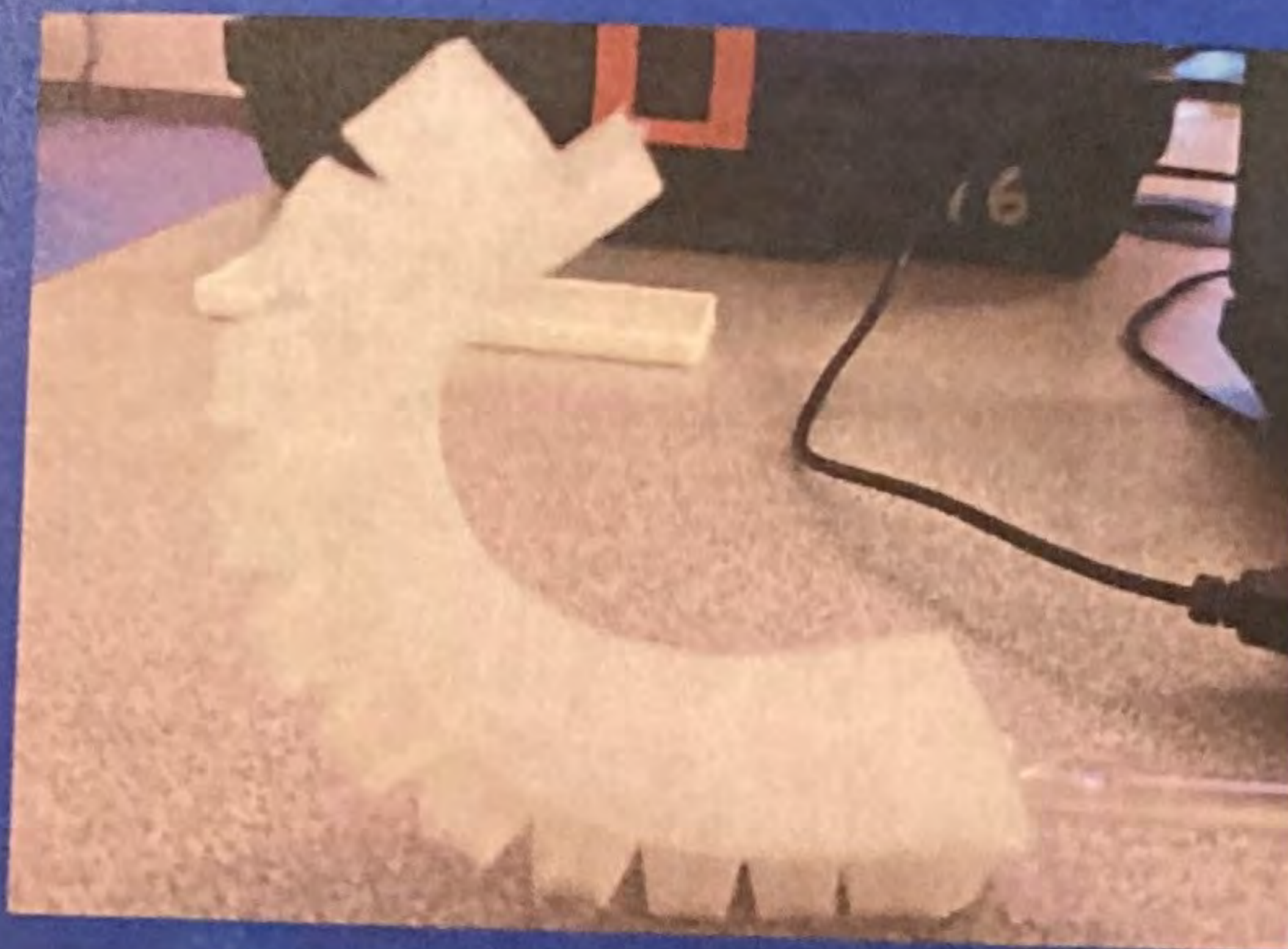
(curling actuator due to air being added)
