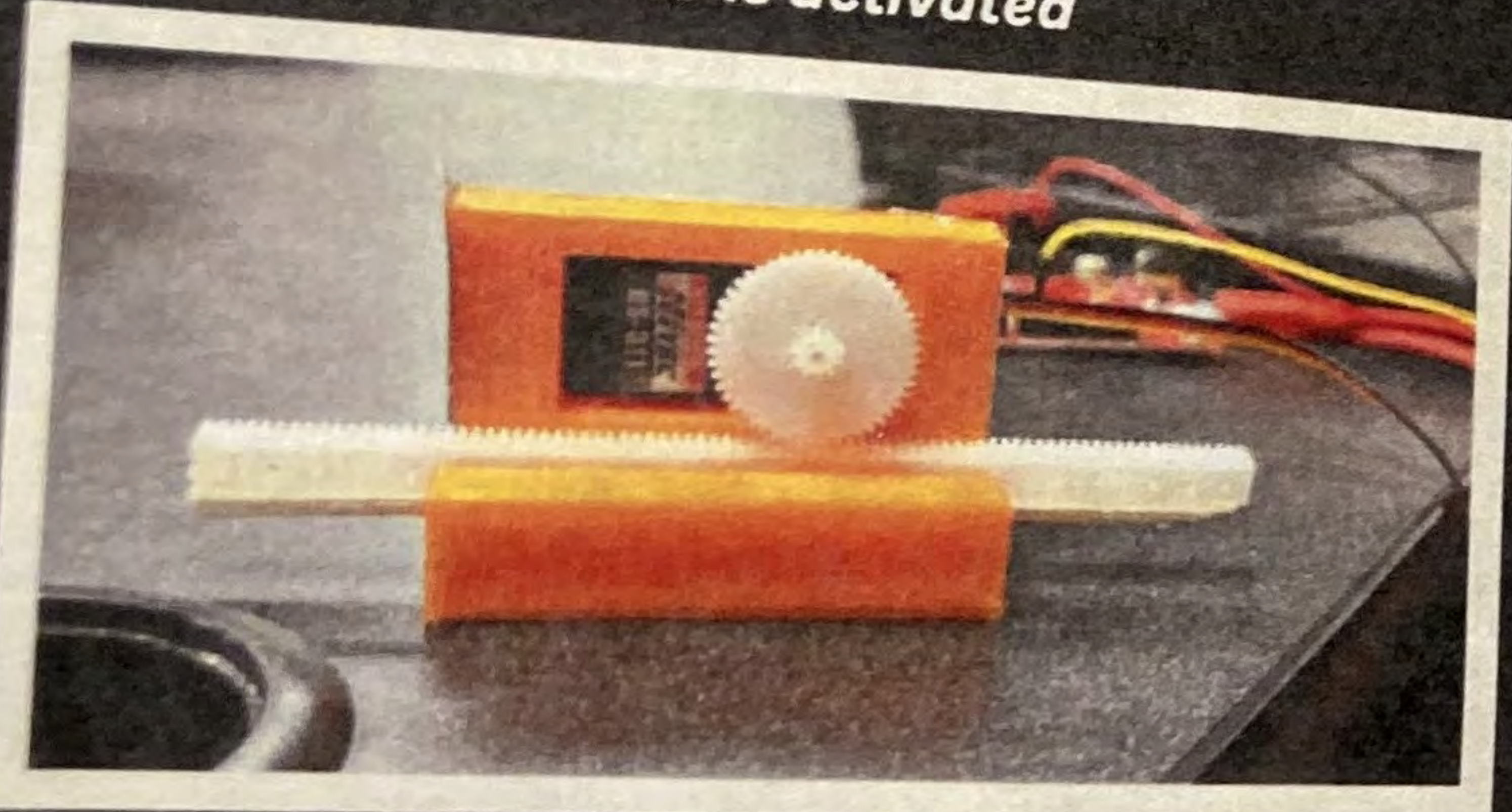
• Gear teeth connecting rod with modified gear. When the servo button is pushed, the gear will retract the rod, pulling the syringe back, creating a suction
