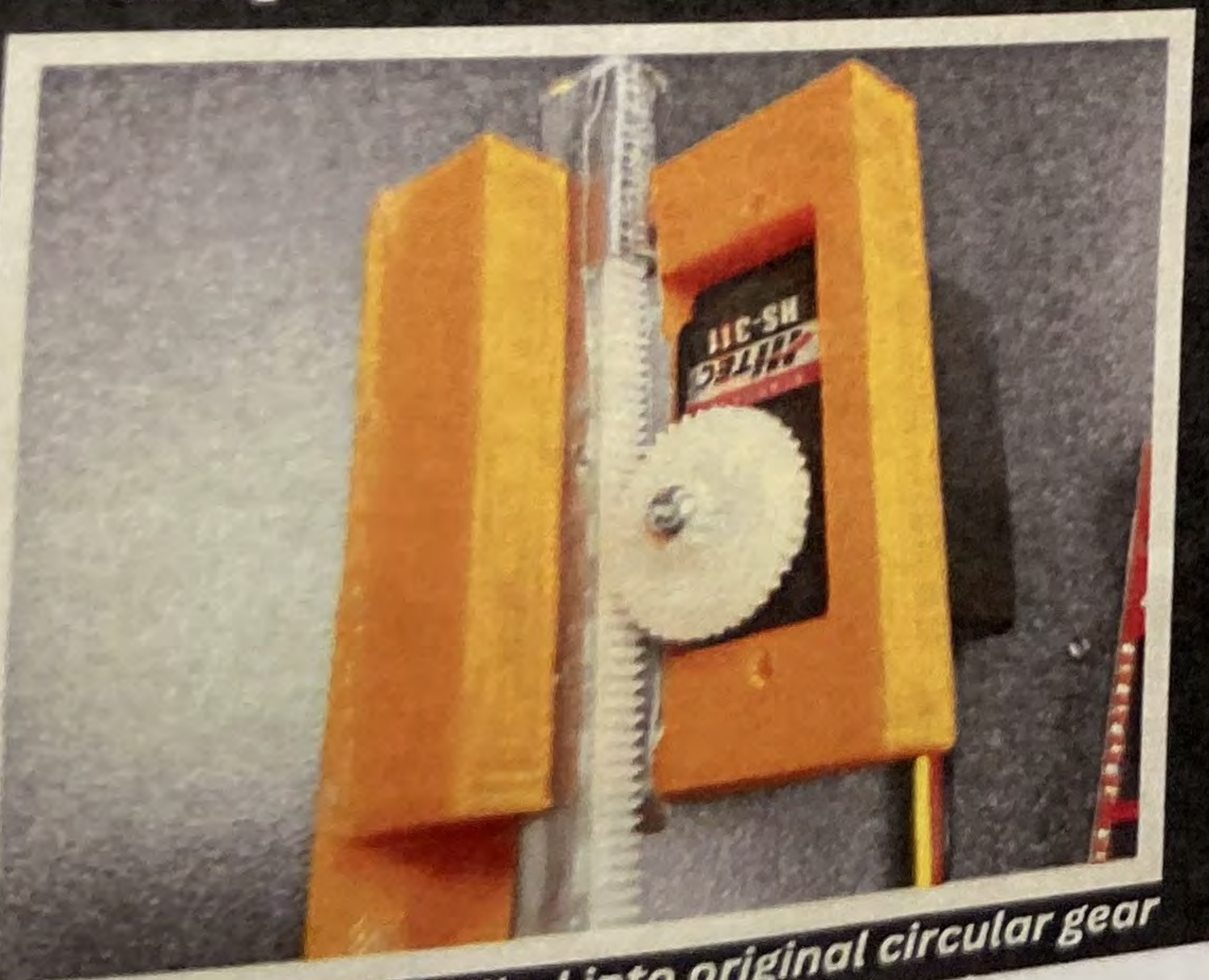
• Gear teeth connecting rod with modified gear. When the servo button is pushed, the gear will retract the rod, pulling the syringe back, creating a suction
