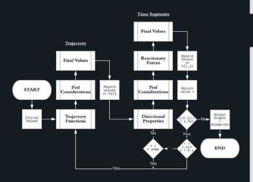
By utilizing nested iterative calculations, the Interactive Resource Impact Simulation is able to successfully predict the trajectory of launched supply pods above and across the surface as well as their spin, temperature, deformation, kinetic energy, and other physical reactions.
