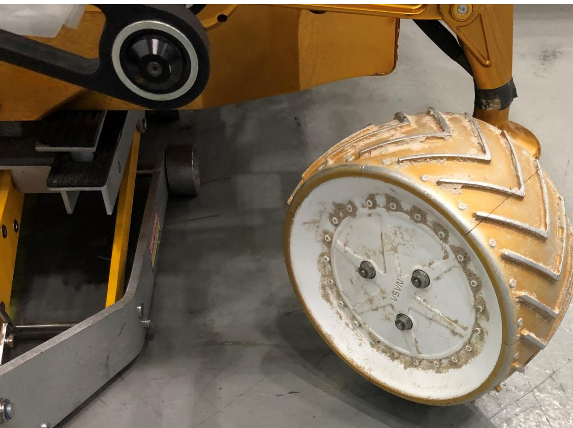
Rover wheel that was tested in the JSC Mars yard.
