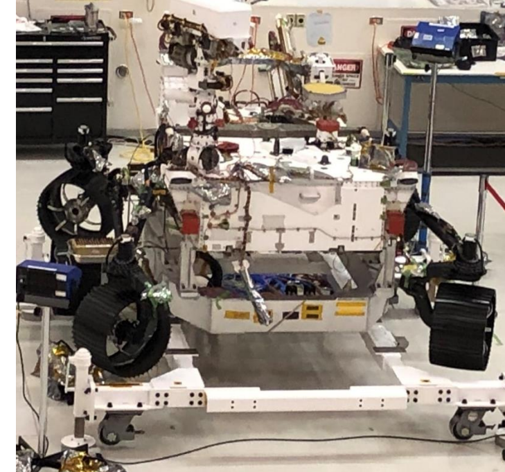
Mars 2020 Rover being assembled at JPL
