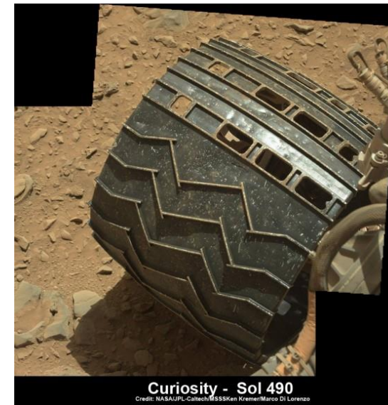
Curiosity Rover wheel on Mars. The angles were determined to cause stress in the aluminum.
