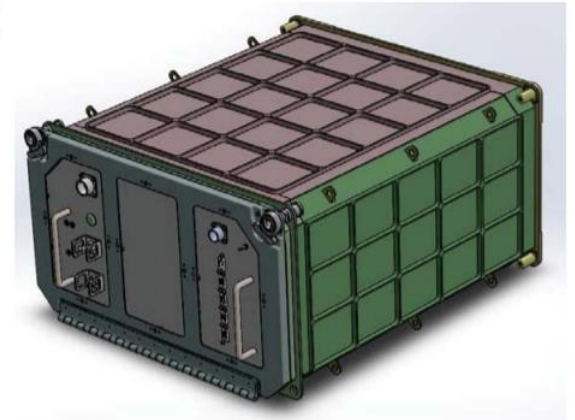
Figure 3-2: Nanoracks Nanode (Mainframe) Assembly Installed in ISS Locker
