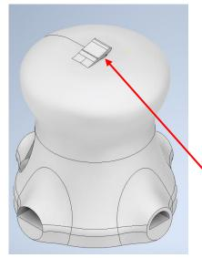
Flapper valves to control the exit airflow and the entrance airflow?
