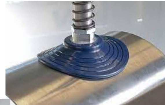
Needs to be able to attach to curved smooth surfaces. Smaller suction cups can attach to curvier surfaces.
