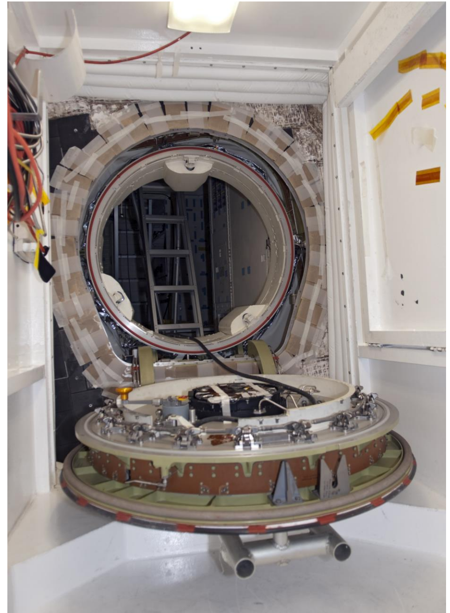
This is the side hatch of the Space Shuttle. This one also had to open outward and hold pressure inside.
