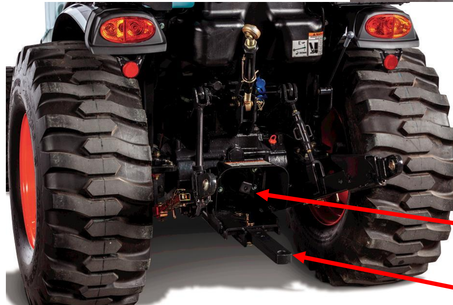
Power Take Off (PTO) – drive shaft from engine to power other equipment
