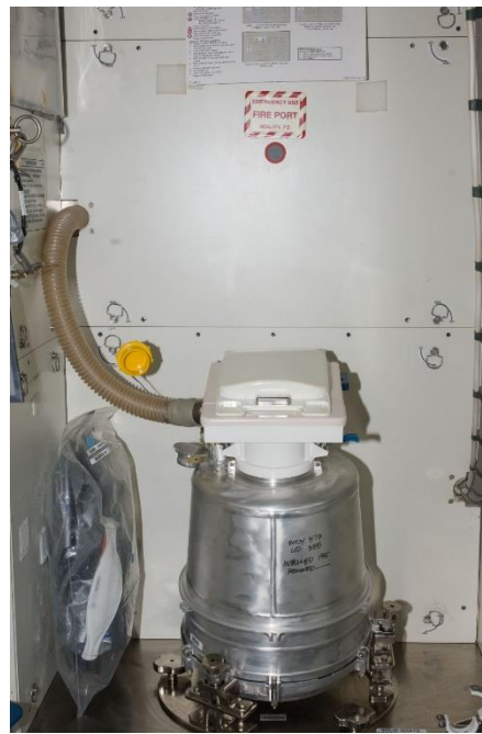
KTO with seat and air hose attached.
